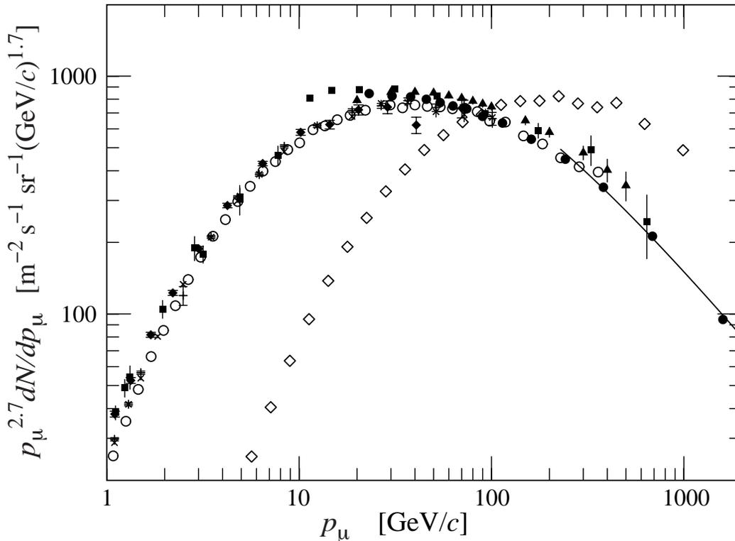
**Figure 30.6:** Spectrum of muons at  $\theta = 0^\circ$  ( $\blacklozenge$  [67],  $\blacksquare$  [71],  $\blacktriangledown$  [72],  $\blacktriangle$  [73],  $\times$ ,  $+$  [69],  $\circ$  [61], and  $\bullet$  [70] and  $\theta = 75^\circ$   $\diamond$  [74]). The line plots the result from Eq. (30.4) for vertical showers.
