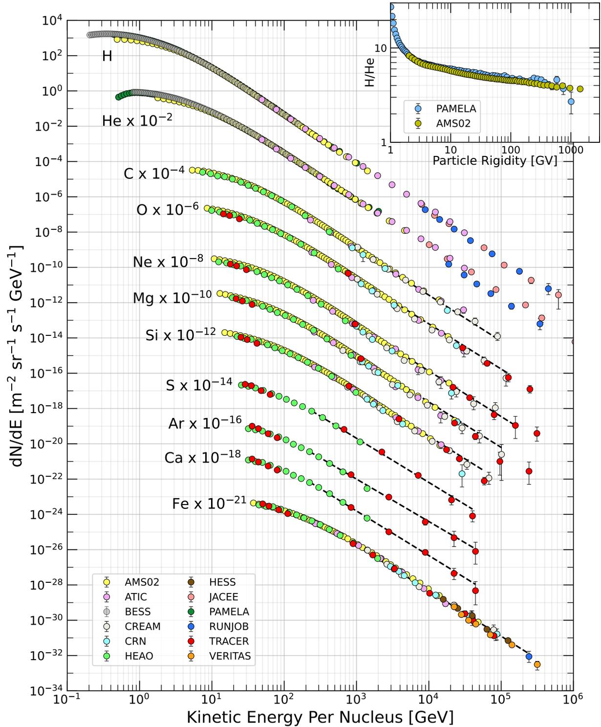
**Figure 30.1:** Fluxes of nuclei of the primary cosmic radiation in particles per energy-per-nucleus are plotted vs energy-per-nucleus using data from Refs. [1–15] The inset shows the H/He ratio as a function of rigidity [1, 3].
