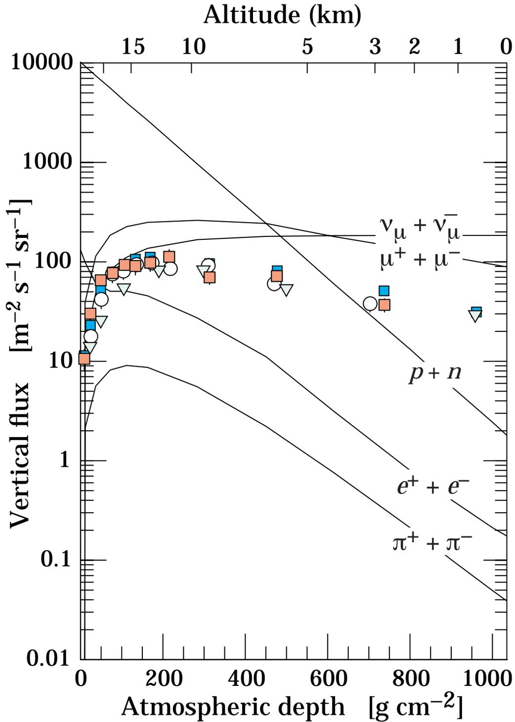
**Figure 30.5:** Vertical fluxes of cosmic rays in the atmosphere with  $E > 1$  GeV estimated from the nucleon flux of Eq. (30.2). The experimental points show measurements of negative muons with  $E_\mu > 1$  GeV [56–61].
